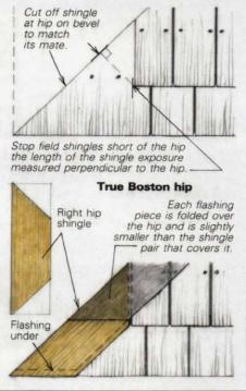
A true Boston hip, shown at left in a model built by Syvanen, uses the hip shingles to complete each course. The usual way is to superimpose a line of ridge shingles on the hip. The butts of Boston hip shingles can run parallel to the eaves, as shown on the right side of the model, or perpendicular to the hip (left side).
