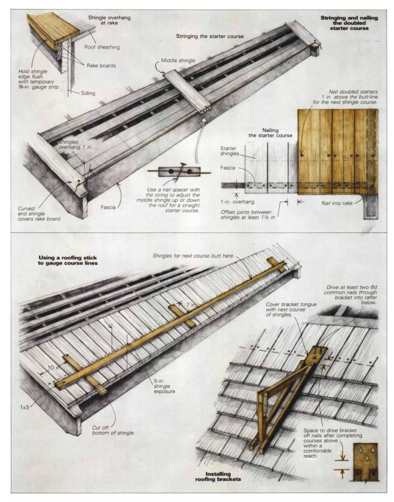
When using roof brackets, or jacks, squatting is usually the most comfortable working position. Once you have shingled up the roof to a point where you are working at full arm extension, nail a new line of brackets to the rafters higher up the roof. These brackets are removed when the roof is completed by tapping them at the bottom. The 8d common nails used to secure each bracket remain under the shingles.
