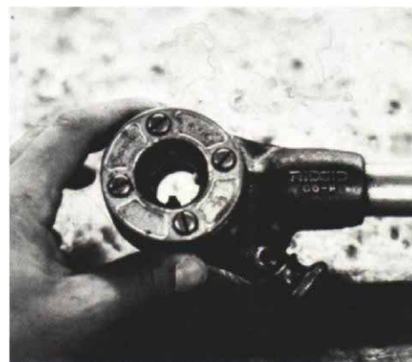
A ratcheted pipe threader needs only 1\frac{1}{4} in. of clearance around the pipe, making it ideal for threading pipe in place. For extremely tight spaces, the handle can be replaced with a short section of \frac{3}{4} -in. threaded pipe.
