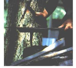
*Traditional tools.* The slater's stake is T-shaped, and its sharp end can be driven into a rafter or other wood work surface. Its horizon-tal edge supports the slate while it's punched, cut and smoothed. The hammer, which is made from a single piece of drop-forged steel, is designed to drive and pull roofing nails, to punch holes and smooth the rough edges of cut slate.
