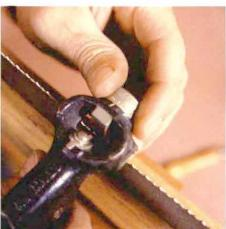
**Setting.** A saw-set is used to bend the top half of the teeth alternately to the left and right. As shown above, the plunger pushes on the saw tooth, forcing it against the anvil each time the pistol grip of the handle is squeezed. All saw-sets are adjustable for width of set. A handsaw used mostly on wet lumber should get a wider set than one used mostly on dry wood to reduce friction on the blade and to evacuate the moist sawdust more easily.
