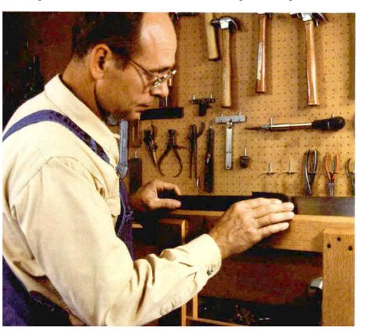
will start the cut. Push the saw lightly forward to cut a little deeper. Now move your thumb away; too much pressure on the first few strokes may cause the saw to jump out of the kerf, leaving you with some lifetime scars.
