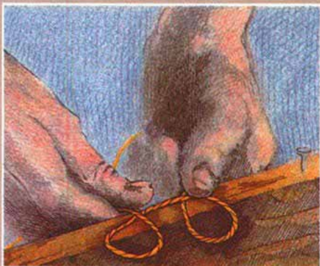
1. Form two consecutive underhand loops in the standing part of the line.
