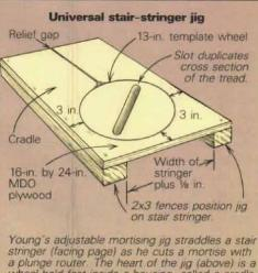
roung s adjustable mortising jig straddles a stair stringer (facing page) as he cuts a mortise with a plunge router. The heart of the jig (above) is a wheel held fast inside a housing, called a cradle. The wheel adjusts to any stair layout, and the entire assembly is secured to the stringer with a bar clamp and a pair of shim shingles.
