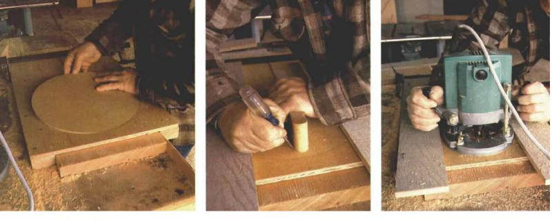
*Making the template.* To cut the template, Young first draws a centerline through the wheel, left, and aligns it parallel with the long edges of the brake. Next he tacks a pair of parallel fences to the cradle to guide the router as it cuts the template. Young uses a section of the tread material to scribe its dimensions onto the wheel, center. Then he routs freehand to the scribe marks, right.
