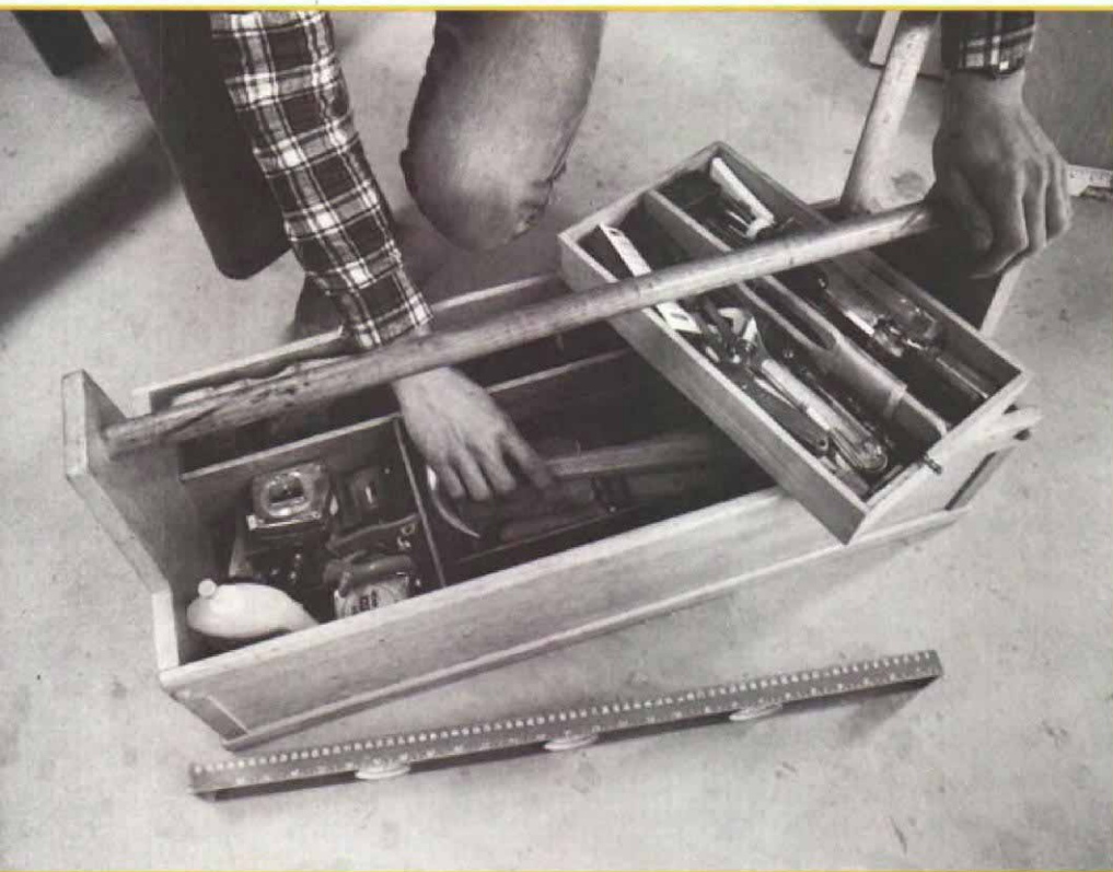
Long and narrow, the open shoulder box has traditionally been the workhorse toolbox of the framing carpenter. Elaborate versions, like the one shown above, are divided into compartments to keep edge tools or delicate tools like handsaws and levels separate from the jumble of tools below. Portable and rugged, this type of toolbox has two main disadvantages: It offers no protection from sawdust or bad weather, and tools often have to be hunted for.
