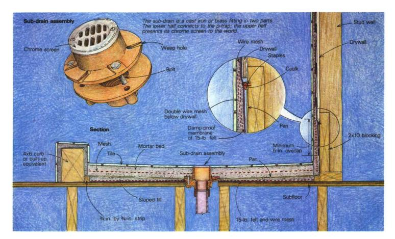
antee. In addition, companion sealers, caulks and accessory patches (preformed corner pieces) enable me to create shower pans in any shape. Chloraloy 240 (The Noble Co., 614 Monroe St., Box 332, Grand Haven, Mich. 49417) is the brand I use, with no failures on over 600 pans. A similar product is called Composeal 40 (The Compotite Corporation, PO Box 26188, Los Angeles, Calif. 90026).
