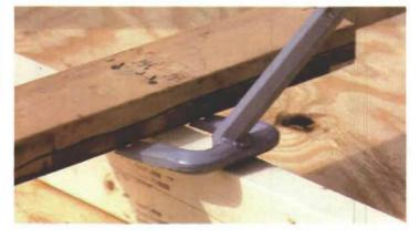
first-class levers, the fulcrum (or pivot point) is between you and the load, or the nail you are pulling. This is the leverage you get with hammers and other tools with claws at  $90^{\circ}$  to the handle. The second-class lever has the load between you and the fulcrum. This is the kind of leverage you get when you pull up on tools with nail slots in the handle.
