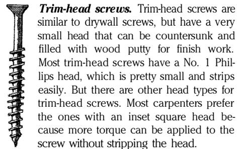
**Trim-head screws.** Trim-head screws are similar to drywall screws, but have a very small head that can be countersunk and filled with wood putty for finish work. Most trim-head screws have a No. 1 Phillips head, which is pretty small and strips easily. But there are other head types for trim-head screws. Most carpenters prefer the ones with an inset square head because more torque can be applied to the screw without stripping the head.
