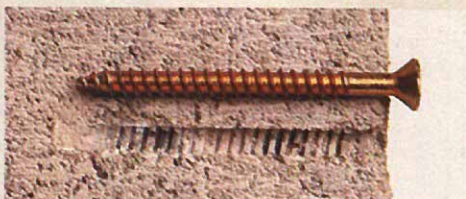
Concrete screws work like woodscrews. After drilling a pilot hole (top), the drill bit is retracted into the shaft of the installation tool, a Phillips-head bit is inserted and the screw is driven into the hole (middle), cutting its own threads in the concrete (bottom).
