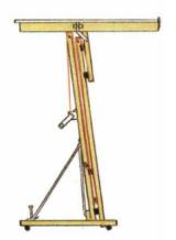
Next, with the mast lock engaged, the cradle is winched up to the top of the masts. The cradle pivots on <sup>1</sup>/<sub>6</sub>-in. angle-iron brackets, and is locked in place with the tilt latch.
