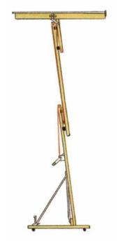
Finally, the mast lock is unhooked, and the drywall is winched up to the ceiling. The lift works for ceilings up to 10 ft. high or, in the horizontal position, for walls up to 77 ft. high
