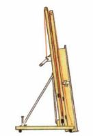
First, the cradle is lowered to the floor in the vertical position. Drywall is then tilted up against the cradle, with the bottom edge of the drywall resting on the support clips.
