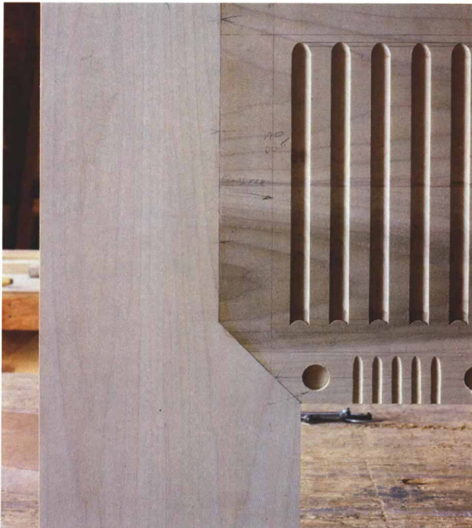
With a shop-built jig and a \frac{5}{16} -in. core box bit in a plunge router, the author cut the vertical flutes that create the frieze under the mantel shelf (photo above). Where the joint would show between the horizontal and vertical members of the frame, the pieces are mitered (photo below). The butted portion will be hidden behind the pilaster. Notice how the ends of the flutes are carved so that they appear to point upward. (Photo below by author).
