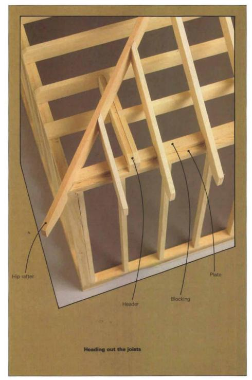
f you want a simple roof, go for a gable. The angles are basic, and even the ceiling framing is a snap because it generally runs parallel to the rafters. A hip, however, is a roof to reckon with, and not just because of its angles. With rafters sloping up from all four sides of the building, how do you joist the ceiling?
