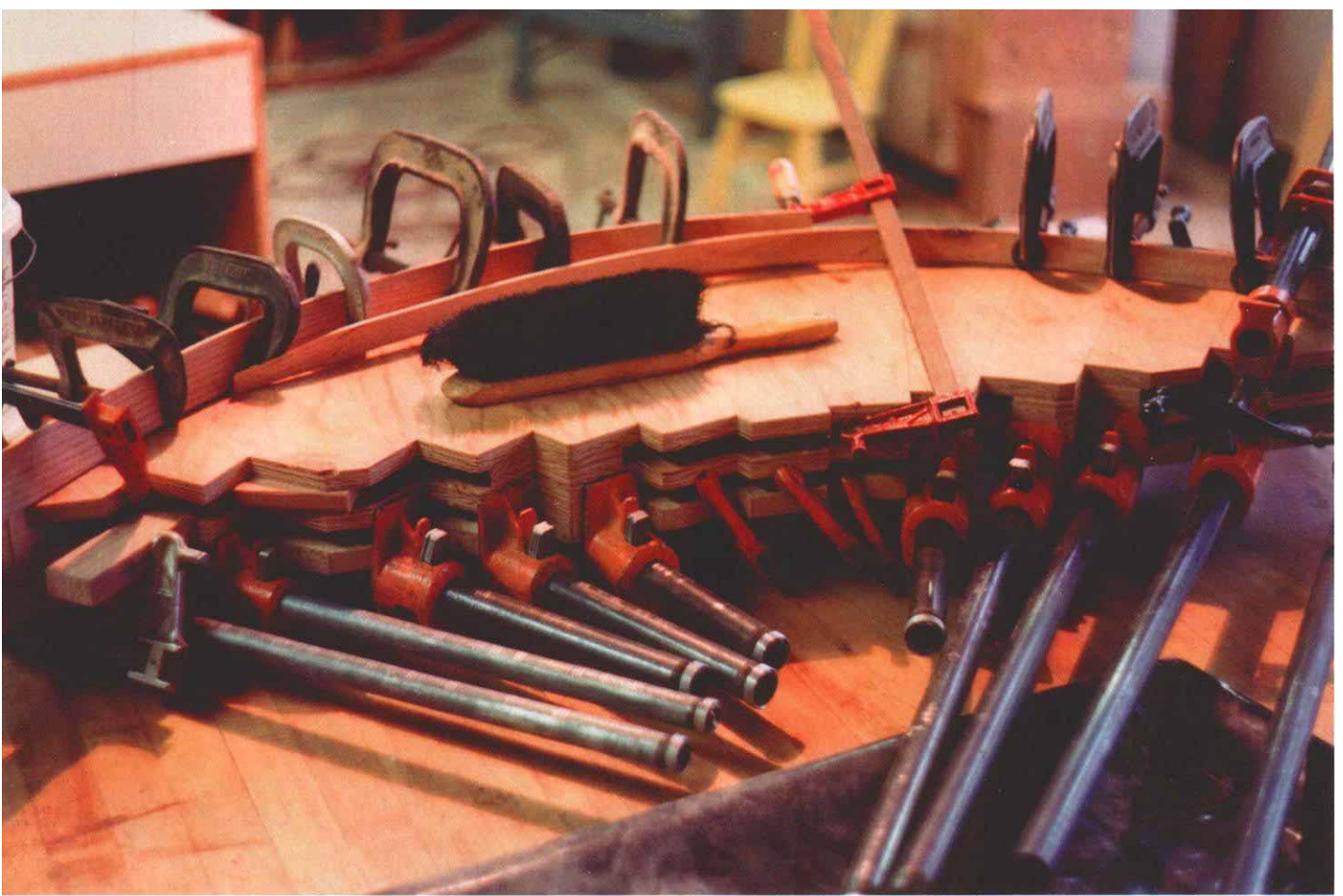
Glue up. The laminating form consisted of three layers of \frac{3}{4} -in. plywood separated by \frac{3}{4} -in. plywood spacers (photo above). A series of steps bandsawn into the back of the form provided solid footing for an assortment of clamps. Extra strips of pine (photo below) placed against the molding stock helped distribute the clamping pressure.
