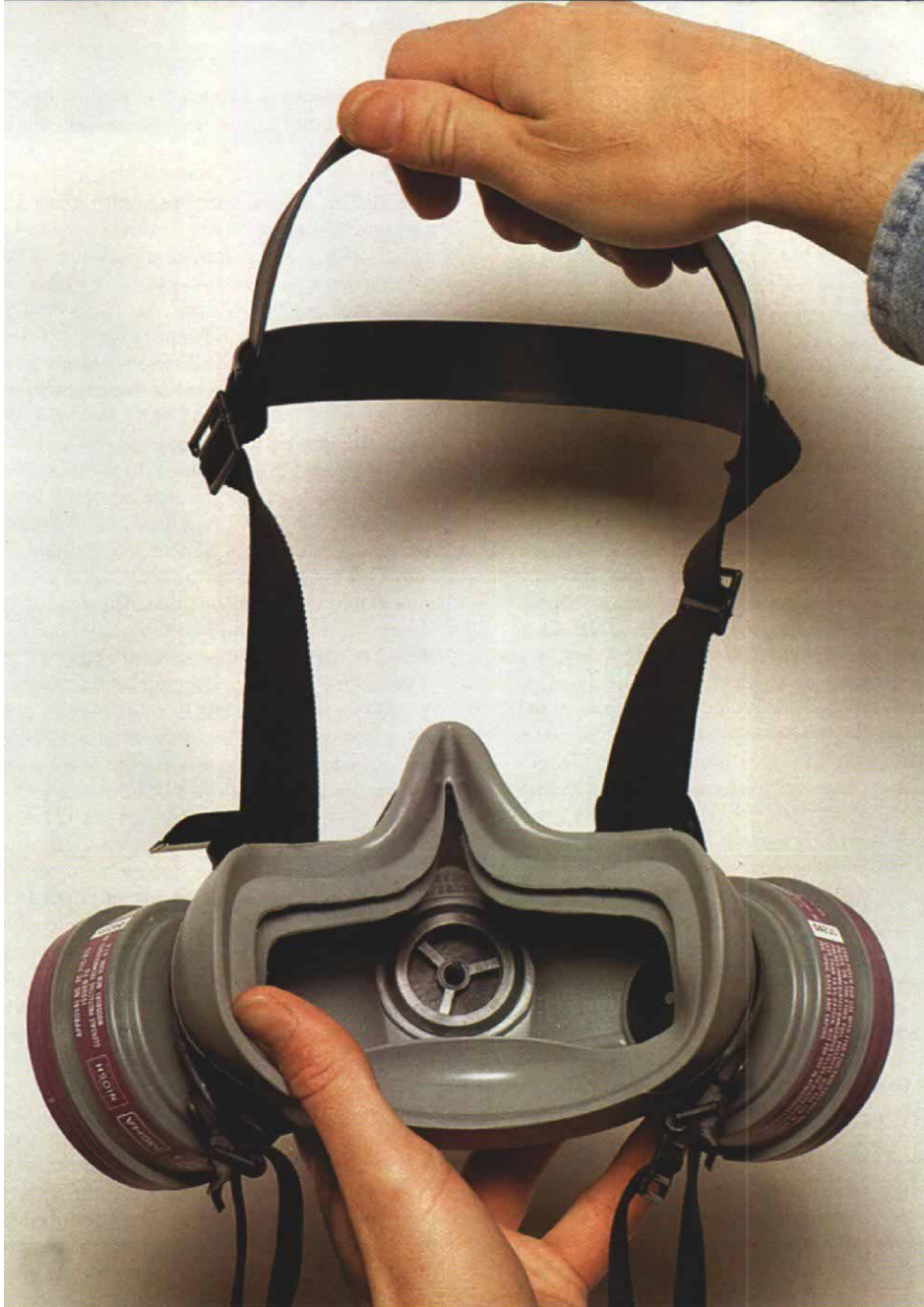
Half-mask respirators. The best half-mask respirators have a yoke-style top strap, which holds the facepiece in place with pressure applied evenly. Some facepieces, such as the one shown above by Glendale Protective Technologies, have a double-seal feature to ensure a snug fit against the face. This rig is outfitted with HEPA filters, which are identified by the magenta stripes.
