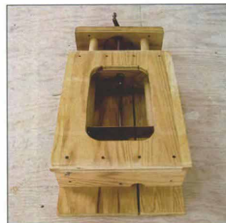
C-clamp vise. Pawlik used the screw mechanisms from large C-clamps to make the vises for the bench's sliding tables. Hardwood dowels serve as guides for the vises' jaws.
