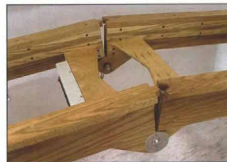
The key to rigidity. A key cut in the 1x3 sub-frame helps register and stabilize the bench's frame when it is open.
