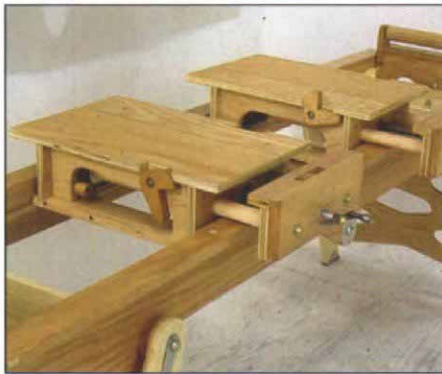
Sliding tables. Both sliding tables ride on oak runners. Each table is equipped with three bench dogs and a vise.
