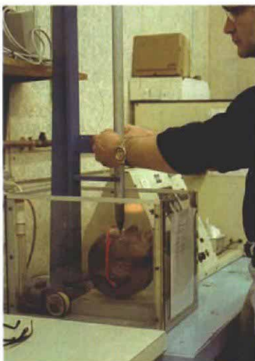
The glasses passed the test. An inspector at a Uvex factory in Smithfield, R. I., tests a pair of safety frames by dropping a pointed weight on the glasses from a height of about 51 in. The lens stayed in the frame, and the frames were undamaged.
