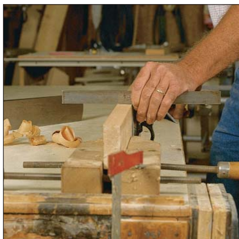
A straightedge must be square as well as straight. After truing the edge with a jointer plane, the author checks for square before applying a wax finish.
