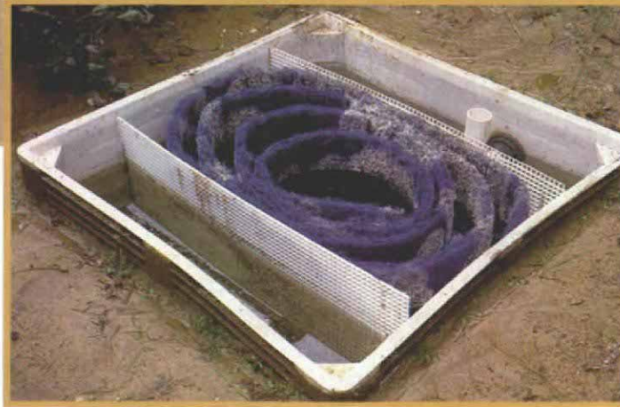
A biological filter. Biological filters rely on organisms to cleanse the water of nutrients such as algae. The organisms live in the filter medium, in this case the fiberglass filter from a forced-air heating system. This site-built filter was made from a fiberglass tank typically used in the agriculture business.
