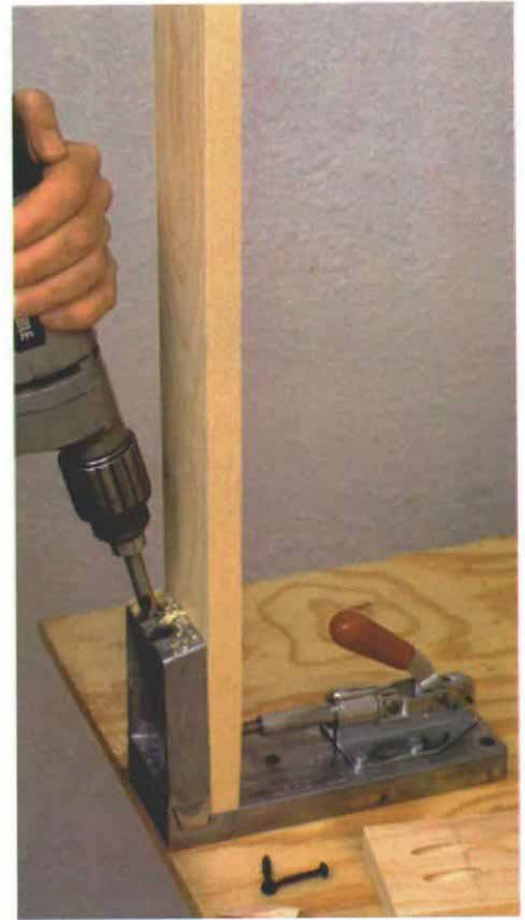
Pocket-screw joinery is fast and strong. Kreg's pocket-hole system joins two pieces of wood with countersunk, self-tapping panhead screws that can be concealed by angled wood plugs. Screw holes (pockets) are produced using a stepped drill bit and an aluminum jig.
