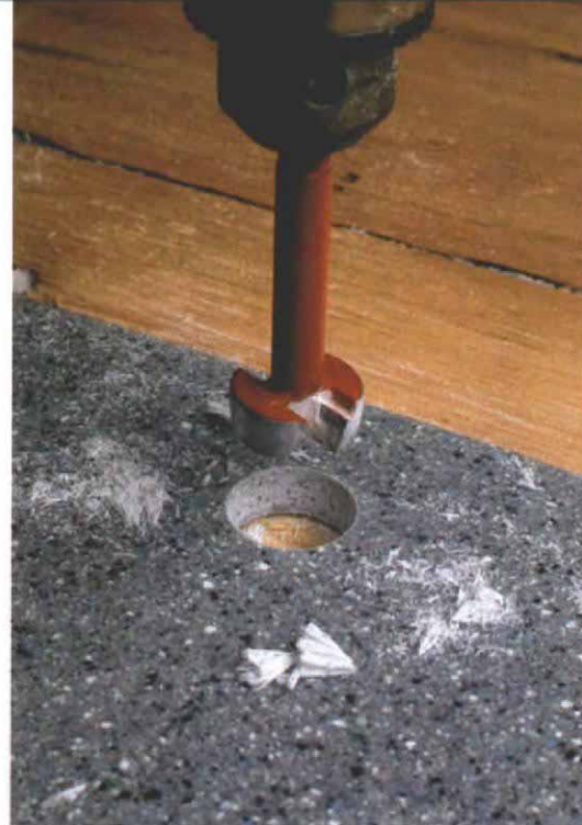
Carbide-tipped Forstner bits bore without overheating. Freud's carbide-tipped Forstners can bore through hard materials such as this Avonite countertop.
