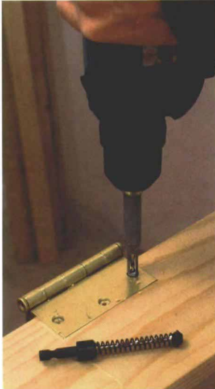
Self-centering bits speed installation. The Vix bit (in drill) centers a twist drill to produce accurate pilot holes. Insty-Bit's Drill Guide (foreground) uses a spring-loaded bushing.
