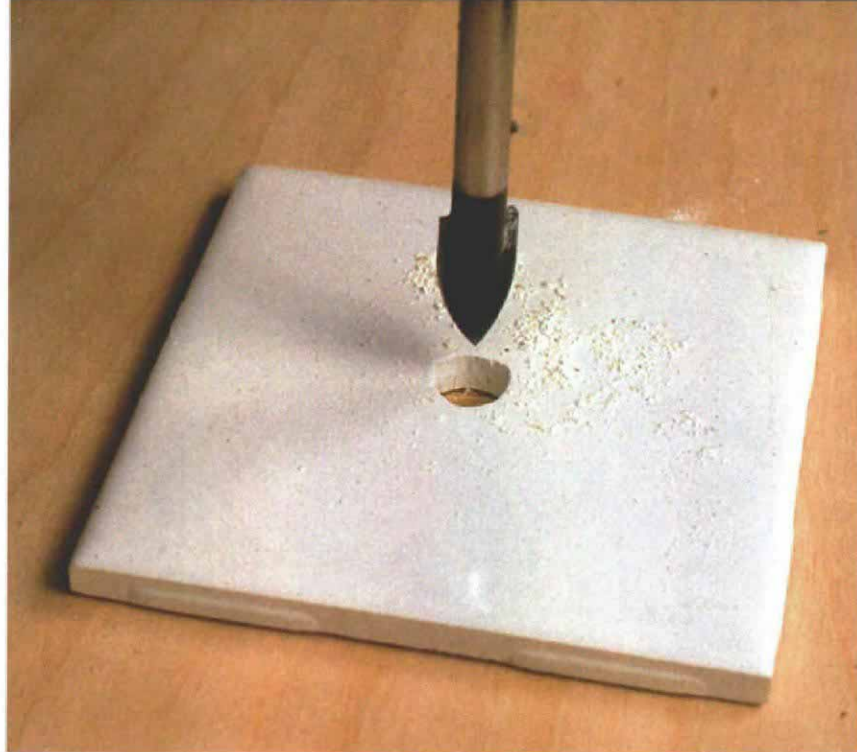
Glass-and-tile bits take on bathrooms. Black & Decker's carbide-tipped glass-and-tile bit chews holes up to 1/2-in. dia. through tiles and mirrors to make way for screws and hollow-wall anchors.
