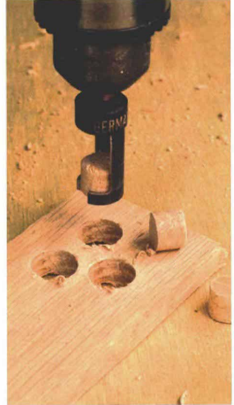
Plug cutters make custom wood plugs. Irwin's self-ejecting plug cutter makes unchamfered plugs of a consistent thickness, then spits out the plugs.
