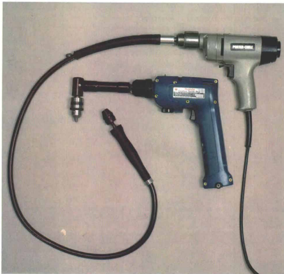
Accessories can reach the tight spots. The 52-in. long flexible extension shaft (chucked in gray drill) by wolcraft snakes around obstacles to drill holes and drive screws. Trendlines' sturdy right-angle drilling attachment (chucked in blue drill) swivels 360°.
