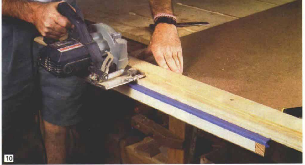
A site-built tool speeds the cut. The author cuts doors with a "shooting stick," a plywood straightedge that has a fence against which he registers the table of his circular saw (10).
