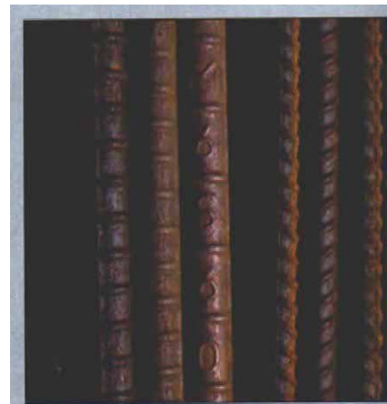
Good information right on the bar. The M signifies the mill that made the steel; the 6 means it's #6 rebar; the S means it's made of new billet steel (the type normally found in rebar); the 6 and 0 mean its yield stress is 60,000 psi.
