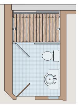
$\frac{1}{2}$ -in. tempered glass. At 5 ft. by 9 ft., this bathroom is not big (drawing facing page). The transparent wall makes it seem spacious.
