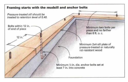
comes in contact with concrete that contacts the ground. To know if lumber has been treated to level 0.40, read the grade stamp on the lumber or the tag stapled to the lumber. (For more on grade stamps, see *FHB* #103, pp. 70-73.)
