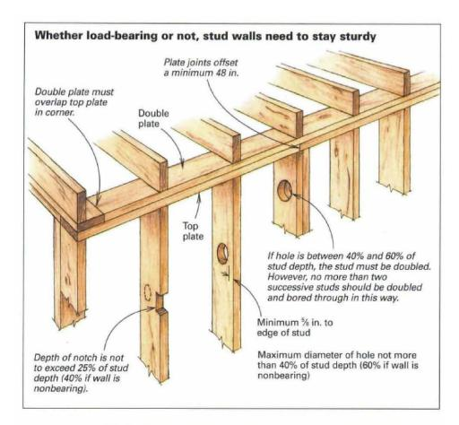
Supporting rafters, joists and trusses with standard stud-frame construction. Top plate, stud size and spacing affect the location of rafters, joists and trusses above.
