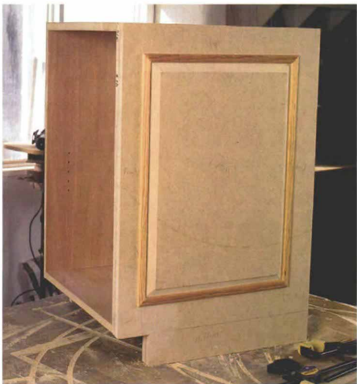
Applied end panel is easier. Rather than integrate the MDF frame and panel into the cabinet construction, the author builds a plywood carcass and screws the MDF frame and panel to it.
