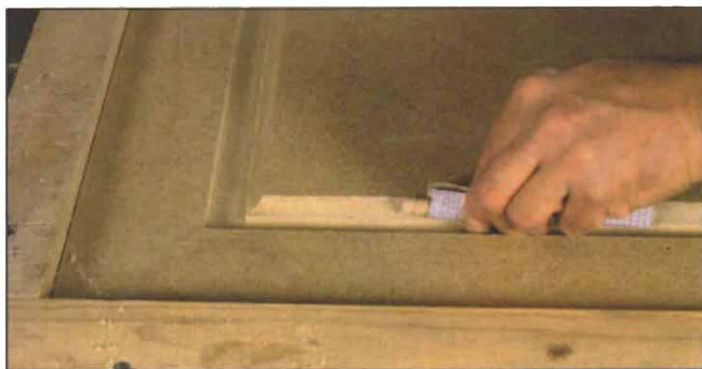
Sandpaper smooths the routed profile. The groove in the door has nearly square corners made with a \frac{1}{4} -in. dia. flush-cutting router bit.
