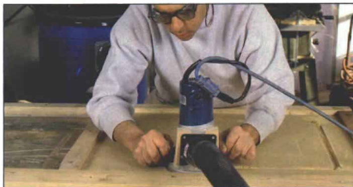
Routers turn MDF into cabinet door. Straightedge boards hold the panel in place and serve as guides for the routers.
