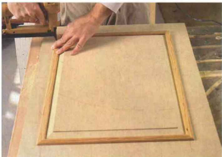
Pine trim covers the gap between the frame and the panel. The cabinet's panel is trapped between the trim on the front and the biscuits on the back.
