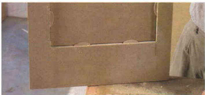
The back doesn't have to be pretty. This frame-and-panel assembly will be attached to the side of a cabinet, so its unfinished appearance on the back will be hidden.
