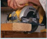
The biggest blade. With a 5½-in. blade, DeWalt's cordless circular saws give greater depth of cut than other cordless circular saws.
