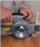
Handy for quick plumbing jobs. The only metal-cutting saw of the bunch is Panasonic's cordless circular saw.
