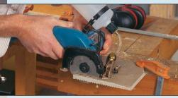
Cut a piece of tile without an elaborate wet-saw setup. Makita's tile- and glass-cutting saw feeds water over the workpiece to keep the blade cool.
