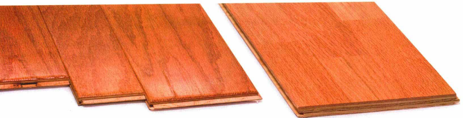
Prefinished engineered flooring. Anderson's engineered flooring (left) is made as single boards with eased edges to hide slight differences in thickness. Harris-Tarkett's LongStrip flooring (right) is made from multiple pieces of veneer laminated to a single substrate.
