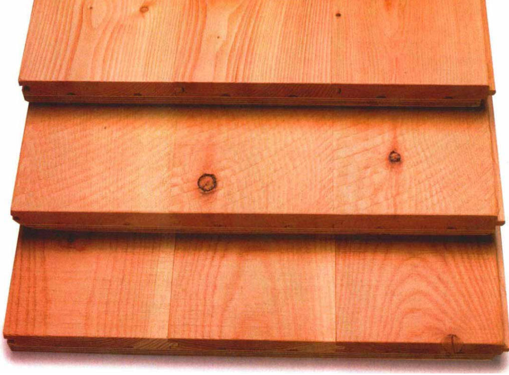
Adding texture at the factory. Country Classics predistresses its fir flooring by adding various textures after the flooring is milled. The top sample has been wire-brushed, which removes some of the softer wood, leaving the grain raised. The bottom two samples have saw marks left in the wood to give the floor a rough-sawn look. Note: The solid-plank flooring was mounted on plywood for display purposes.
