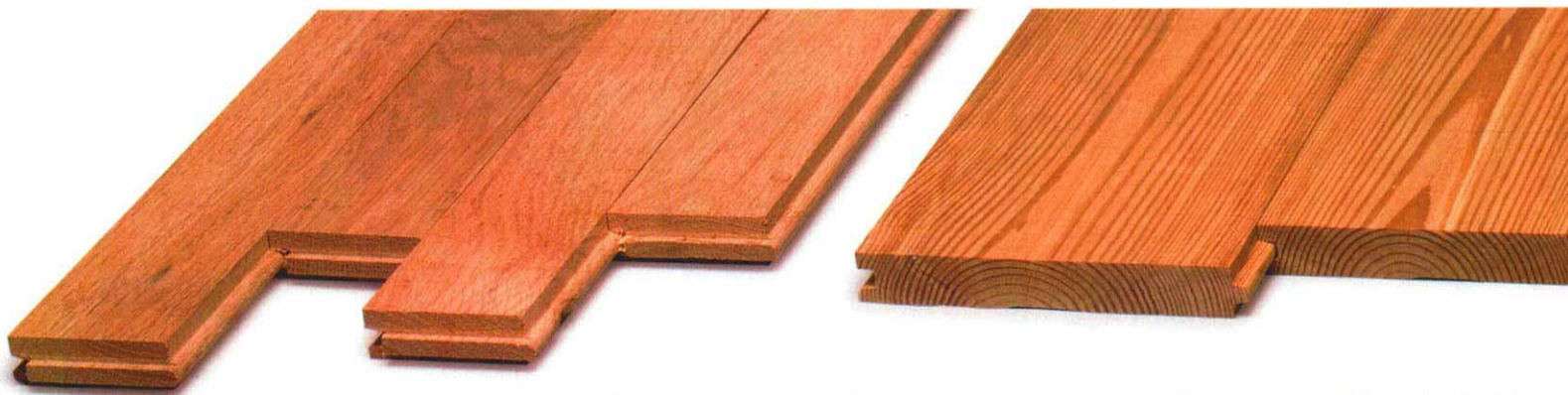
Unfinished solid-wood flooring. Strip flooring (left) is made of solid wood cut to 2¼ in. wide with a tongue and groove milled on the sides and ends. Plank flooring such as the heart pine made by Authentic Pine Floors (right) comes in widths from 4 in. to over 10 in. by special order.
