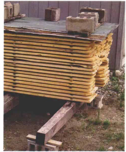
Stacked for air-drying. Strips of wood called stickers separate the layers of freshly cut lumber to allow air to circulate through the stack. Recycled metal roofing covers the pile to keep off the rain and snow.
