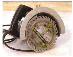
To conceal the expansion gap, the door trim must be undercut with a jamb saw. To hide the necessary  $\frac{1}{3}$  in. expansion gap in places that can't be covered with shoe molding, installers use a special circular saw to cut the door trim at a precise height (photo left). These specialty saws (photo right) have no base plate, and instead bear on the flattened edge of the blade guard. Both the blade's height and cutting depth are adjustable.
