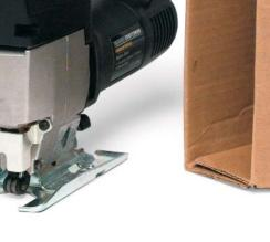
I plunge-cut ¾-in. CDX plywood to see if any saws had a propensity to break blades (photo bottom left). With one exception, the differences seemed to have little to do with saws but much to do with blade style. Uni-
