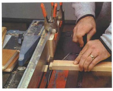
4. Reset the blade for the shoulder cuts. Two passes using an index block clamped to the fence and a miter gauge produce the tenon shoulders. The block prevents offcuts from getting jammed.
