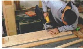
**3. Be careful when cutting biscuit slots.** A biscuit joiner can easily plunge through to the finished side, so a test cut on scrap is a good idea.
