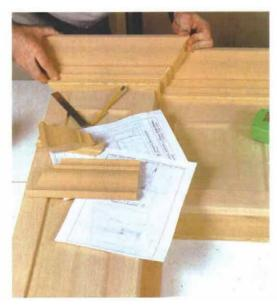
2. Turn it over and add the molding. A narrow piece of 1/2-in. coved stock beneath the lower edge of the crown adds another shadowline. Triangular plywood glue blocks reinforce the top edge of the custom crown molding.
