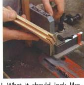
2. Rails get stub tenons. A tenoning I. What it should look like. jig ensures accurate cheek cuts for Cheek cuts should line up with tenons on the ends of the rails.
