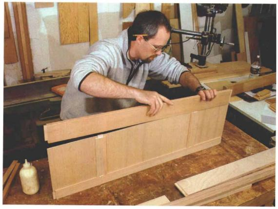
**1. Don't skip the dry fit.** Nothing is worse than gluing up all the parts and then discovering that something doesn't fit, A dry fit gives the author a chance to make minor corrections.
