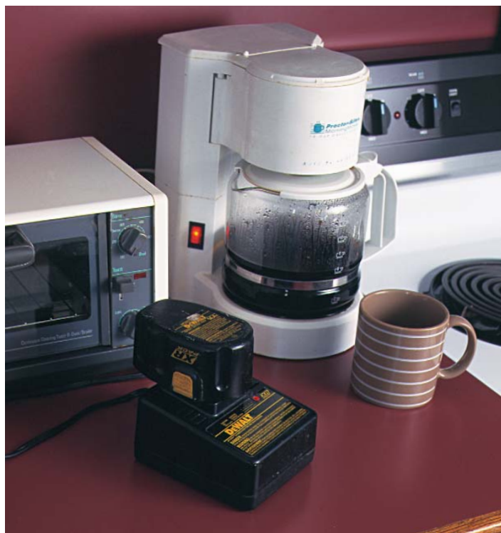
An overnight charge can equalize cells. Because the fast-charge stage might leave some cells partially charged, DeWalt recommends that every tenth charge be about six hours long to equalize the cells.
