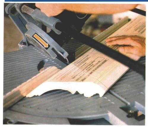
**Wait a minute.** That's upside down. Because the front edges of the molding are manufactured to more exacting tolerances than the backside, the manufacturer of this molding requires that all cuts be made face down.
