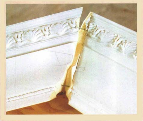
of each other. Getting a mirror image right took some trial and error. We'd make the first cuts a little long, check the fit in the jig and then fine-tune the settings on the saw before making the exact cuts.
