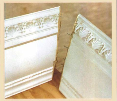
**Don't think you can save money by using the cheap stuff.** As a test, the author glued up one joint using the manufacturer's adhesive and another one with standard construction adhesive. The joint made with standard adhesive (photo above) was easily pulled apart, but the one made with the manufacturer's adhesive was stronger than the molding itself (photo below).
