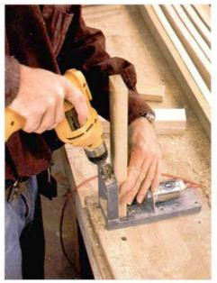
**Pocket-screw jig guides counterboring drill bit at a steep angle.** This jig's clamp is powered by compressed air; similar jigs with toggle clamps are available.
