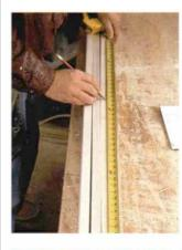
Using a square, the author will extend marks across all the stiles. The rails will butt these marks. Marking several members at once ensures consistent spacing.
