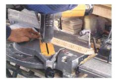
Short pieces of molding are mitered to length using a stop block. This production technique is reliable because the stiles were also cut using a stop block.
