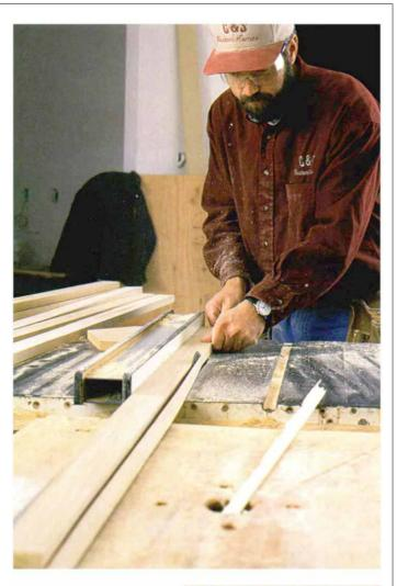
The respective widths of the rails and stiles should be consistent. The exception is in corners, where one panel laps another. Here, the author widens the lapped stile or rail by the thickness of the abutting panel. To guarantee uniform width, stock is ripped slightly oversize, then passed through a planer several pieces at a time.
