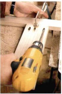
**Locking pliers clamp rail to stile.** Because of their low angle, pocket screws pull the joint together tightly with little movement of the pieces.
