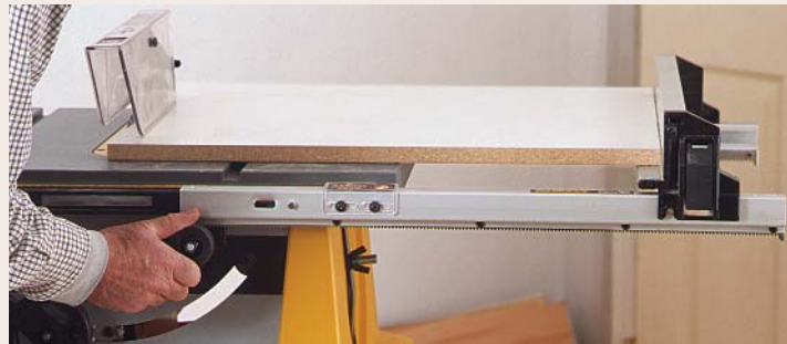
Rack-and-pinion precision. DeWalt's extension-rail system uses front and rear gears that let the operator dial in the proper rip while keeping the fence in perfect alignment.
