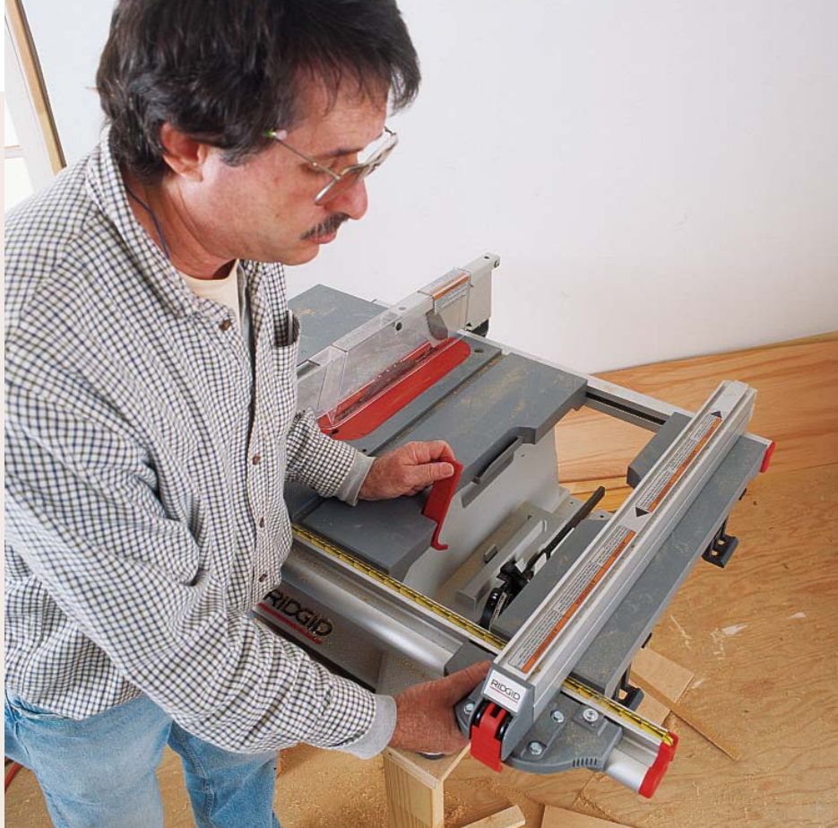
A lever releases the extension table. The fence on the Ridgid saw can slide independently on its rails, or it can lock onto an extension table that is released with a lever built into the tabletop.
