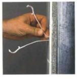
The metal end of the toggle is inserted into a  $\frac{1}{2}$ -in. hole and pulled taut against the back of the stud. A collar slides down the straps and snugs the anchor to the wall. After the straps are detached, the anchor is ready to receive its  $\frac{1}{4}$ 20 bolt.
