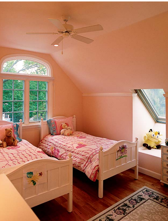
Upstairs bedrooms boast window seats. Bringing the skylights closer to the eaves positioned them where they can serve as roofs for window seats carved into the unused attic space. Photo taken at B on floor plan.
