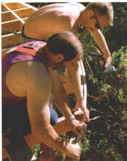
Waterproof glue and staples make quick, reliable laminations. The glue is applied with a disposable paint roller to ensure uniform coverage (photo above). A helper positioning the strips eases stapling them in the correct location (photo right).
