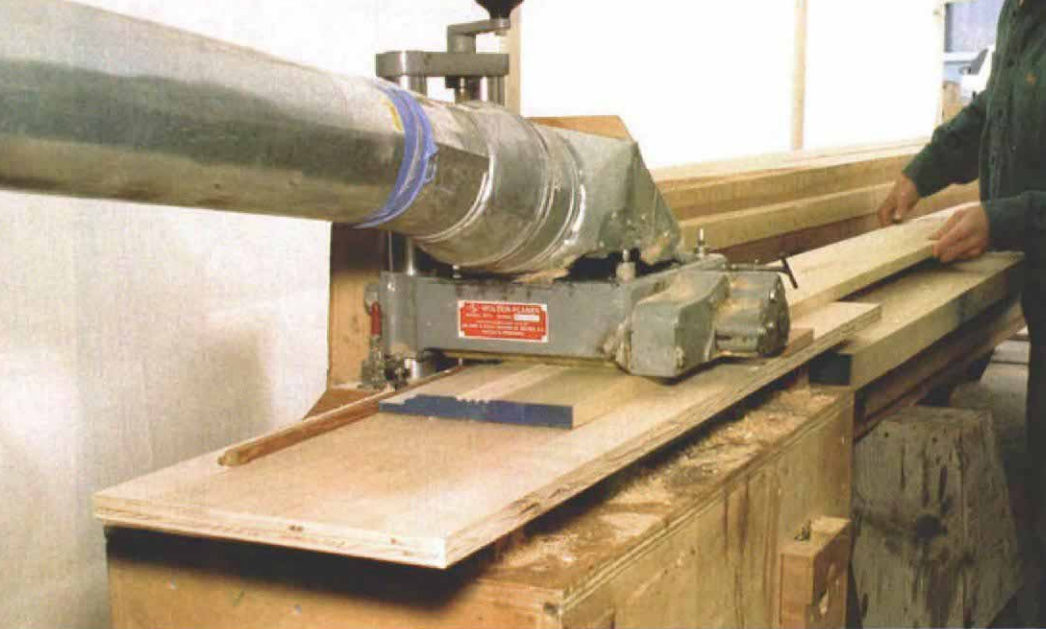
Two passes are better than one. With two sets of knives mounted in a Williams & Hussey molder-planer, the author cuts the baseboard profile in two passes.
