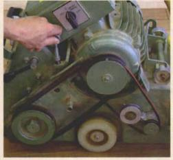
Because belts can take a set and cause bumps in the floor, the sander's drive belts should be loosened with the belt tensioner when the machine is at rest for more than ten minutes.
