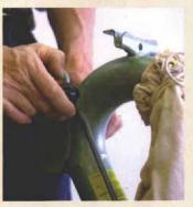
Lever eases drum to floor. The operator needs to drop the sanding drum gradually as the sander moves forward so that the sandpaper doesn't dig a hole in the floor. Before using the machine, practice raising and lowering the drum on a piece of plywood.
