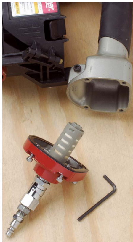
Max and Makita offer on-board air filters that should prolong tool life by blocking grit at the nailer's air intake.
