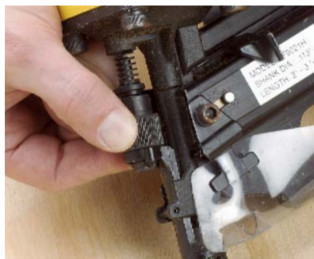
A knurled thumbscrew, as on the Grex (photo above), allows one-handed depth adjustment, while a sliding button mechanism, like that on the Bostitch (photo below), requires two hands.
