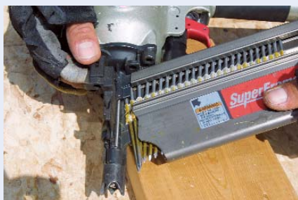
Jam clearing on a stick. Max's SN890RH is the only stick nailer to feature a door for easy jam clearing.
