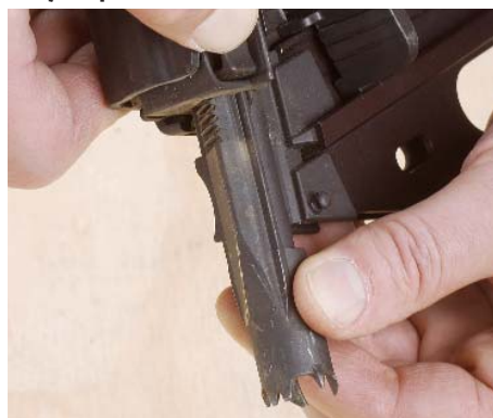
A knurled thumbscrew, as on the Grex (photo above), allows one-handed depth adjustment, while a sliding button mechanism, like that on the Bostitch (photo below), requires two hands.
