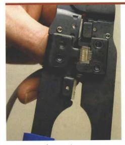
**Crimping in style.** Once the wires are ordered in the jack, this specialty RJ 45 crimping tool squeezes the jack's tiny contacts tight to the wire.
