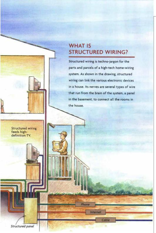
than turbocharged phone wire and coaxial cable. My company installs miles of the stuff. The biggest factor to keeping down installation costs is to get the wiring in before drywall goes up. The cost of doing a structured-wiring system later can be up to four times the cost of installation while the home is under construction.
