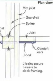
Alignment splines. Wood splines glued and screwed to the sides of each newel post fit into grooves on the sides of the railing sections.
