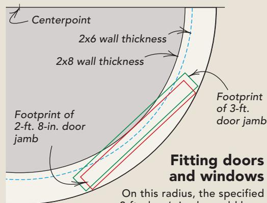
On this radius, the specified 3-ft. door's jamb would have protruded past the inner-wall finish. The fix was to change 2x6 studs to 2x8s and the door to 2 ft. 8 in.
