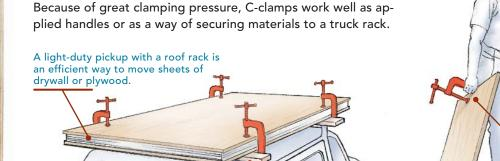
8-in. <u>C-cla</u>mp A C-clamp becomes a handle for pulling plywood up a ladder.
