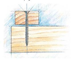
McFeely's ProMax screws come in a variety of unthreaded shank lengths to prevent bridging and overdriving screws to pull the boards together. The differently pitched upper threads of the Spax deck screw pull boards together and lock them in place, aiding the clamping pressure of the head.
