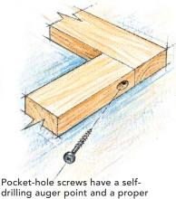
Pocket-hole screws have a selfdrilling auger point and a proper shank length to prevent bridging and speed up joinery-assembly time.
