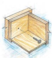
Drawer-front screws have an oversize washer head, allowing a larger pilot hole, which provides room for adjustability.
