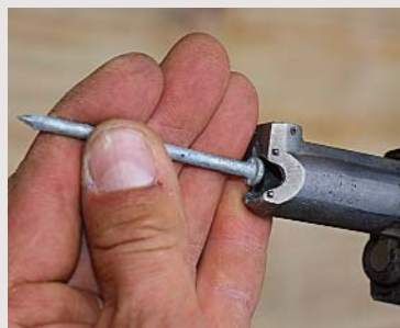
This ultralight gun will drive a 5-in. nail as fast as a framing hammer, without bending it. A simple dial adjustment sets the nail depth so that you don't have to regulate your compressor's psi.
