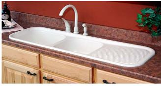
Acrylic is not as hard as some other sink materials, so nonabrasive cleaners are recommended. Surface scratches can be removed with sandpaper, and the gloss restored with car-polishing compound. However, acrylic is susceptible to damage from petroleum-based products and high heat.
