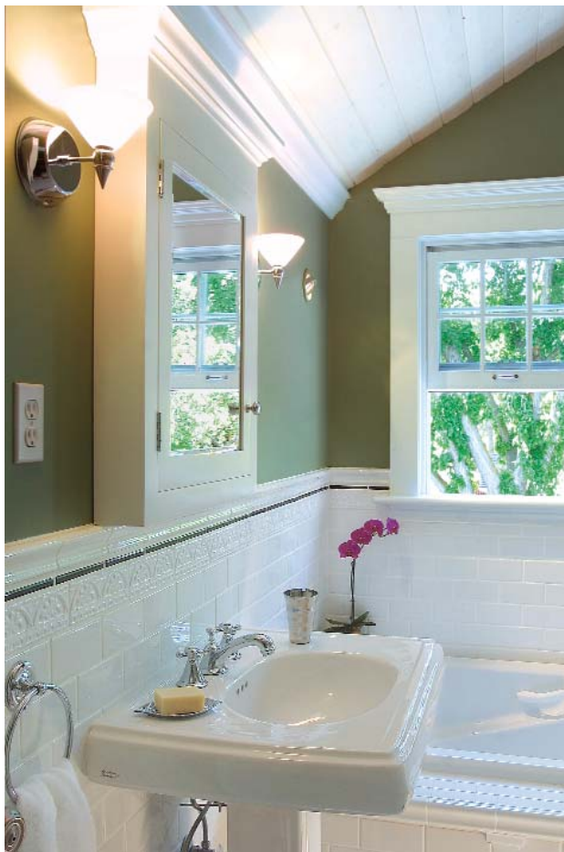
Task lighting is efficient. Sconces flank the medicine cabinet to provide good light for shaving or applying makeup. A spotlight on the wall above the tub makes for shadowless tub-time reading. Photo taken at A on floor plan.
